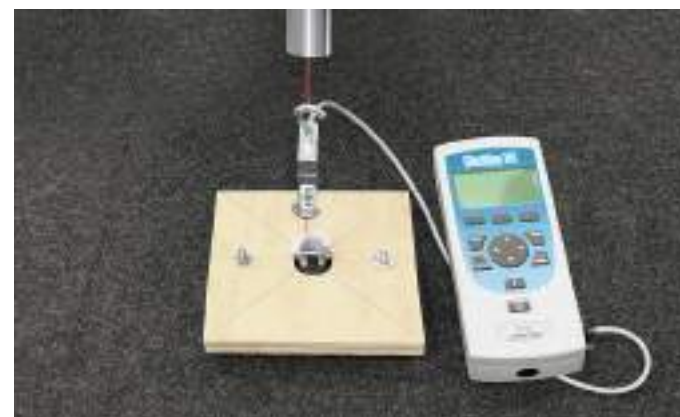
Testing of fixing element strength
