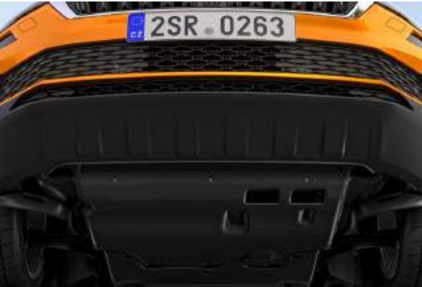
Engine undertray – plastic 57A 071 608E | for TDI 57A 071 608D | for TSI
